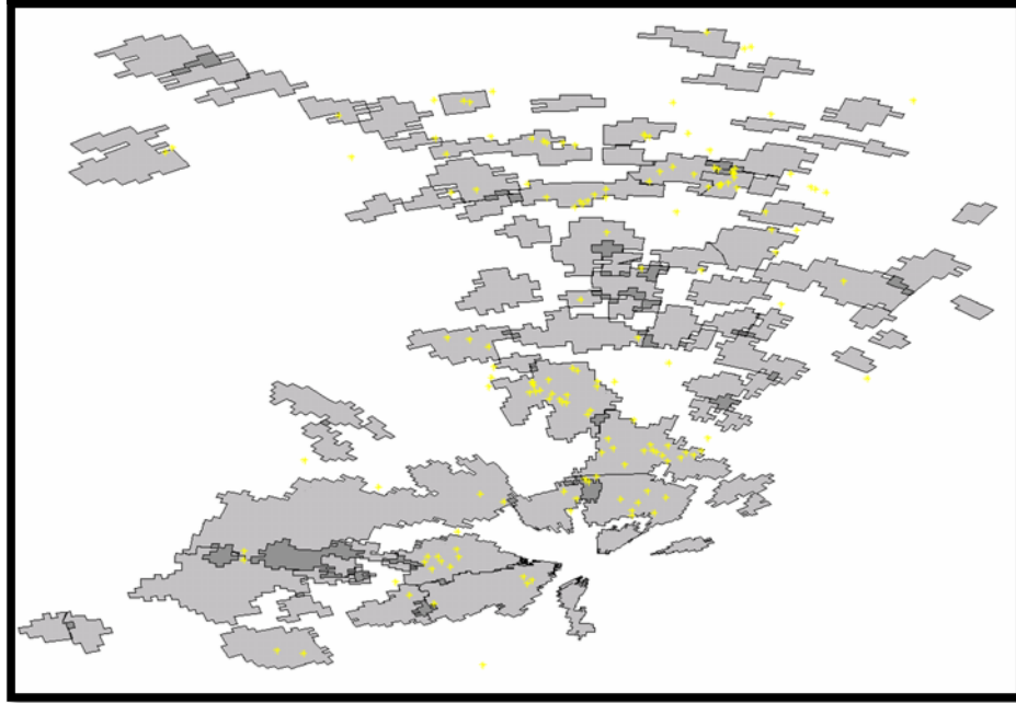
Fig. 10. Map of identified storm cells for a single NEXRAD volume scan and the corresponding lightning strikes that occurred during that scan.
